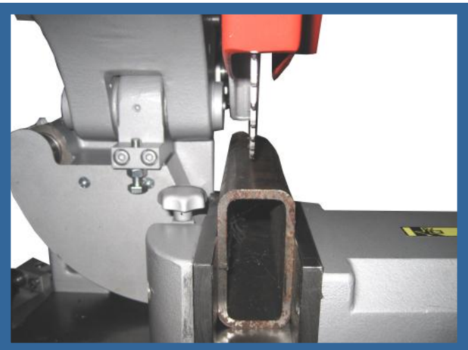
Vise placed for slitting cuts
