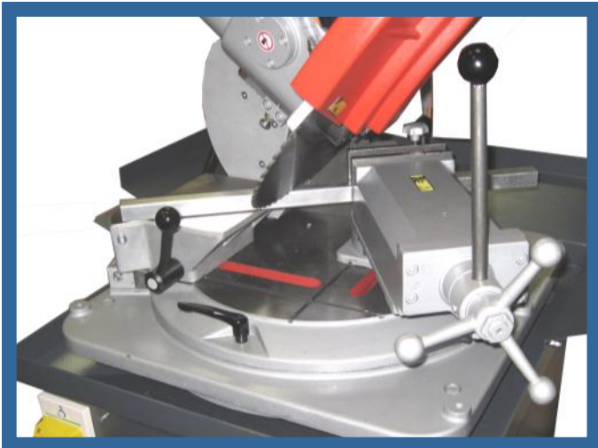
Two-ways mitering for compound angle cuts
