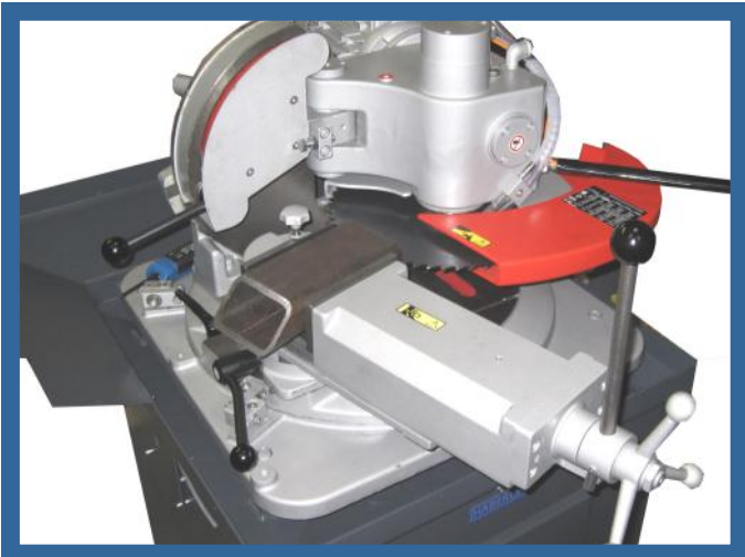
Head tilts 0° - 90° for notching cuts
